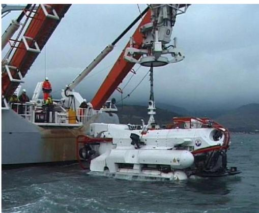
The Portable Launch and Recovery System (PLARS), is a transportable A frame that can be 'attached' to the support ship to enable the SRV to be launched and recovered safely in conditions with wave heights up to 5m
