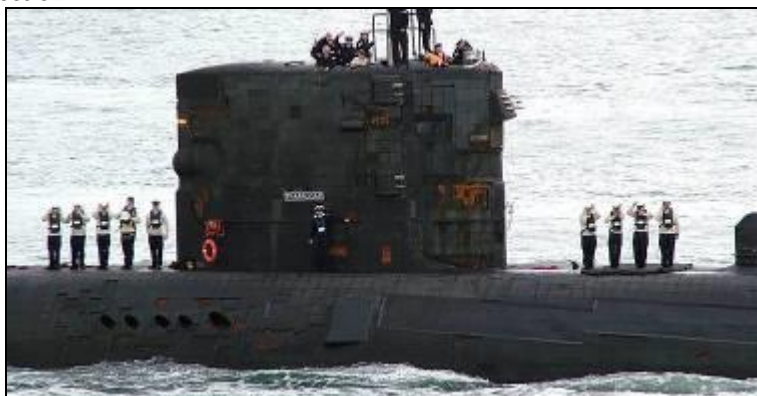
HMS TRAFALGAR entering Portsmouth for a rare submarine visit in August 2006. The 6 probes of the wake detection sensors are prominent on the forward upper fin, with a further 2 pairs on the starboard side. This equipment was fitted at least 15 months before this image was taken.
