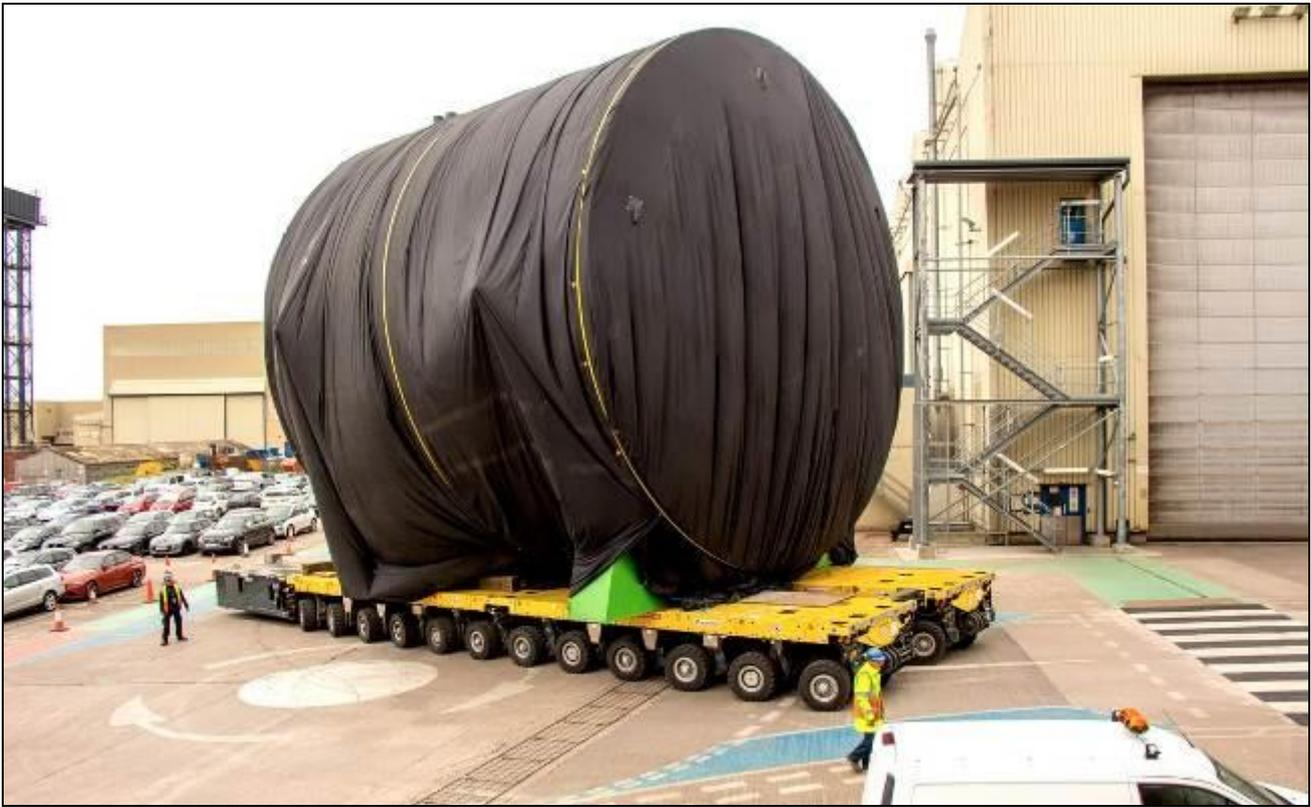
The photo above shows the Accommodation Unit for the new DREADNOUGHT Submarine is seen here being moved across BAE Systems Submarines site in Barrow, where it is being constructed. It is the first unit of DREADNOUGHT's forward end to be moved from the New Assembly Sheds (NAS) into the new Central Yard Facility (CYF). (BAE Tweet 21st June 2019)
